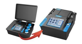
YJS-150 portable particle counter is used to measure the solid particle pollution degree of oil, organic liquid and polymer solution, which can be applied in aviation, aerospace, electric power, oil and other industries.
